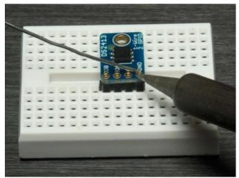
And Solder! Solder each pin to assure a good electrical connection. If you are new to soldering, check out the Adafruit Guide
