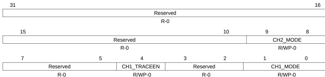
Figure 13-5. CRC Global Control Register 2 (CRC_CTRL2) [offset = 10h]
