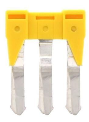
Insulated cross-connector, No. of poles: 3, Mounting type: Plug in, Width: 17.4 mm, Rated cross-section: 4 mm², Colour: Yellow
