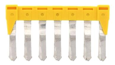
Insulated cross-connector, No. of poles: 7, Mounting type: Plug in, Width: 41.8 mm, Rated cross-section: 4 mm², Colour: Yellow
