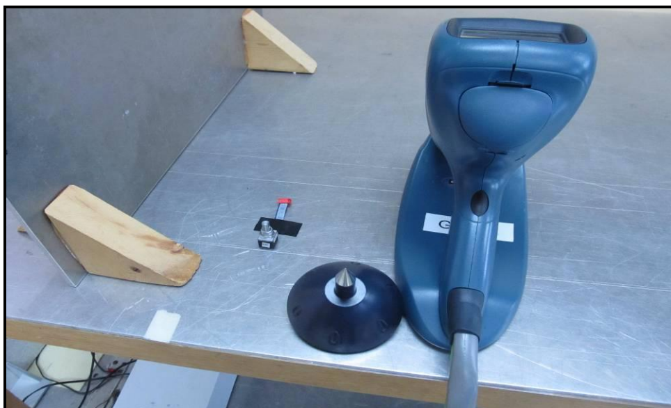
Figure 10 – Electrostatic Discharge Test Setup (Un-Powered)
