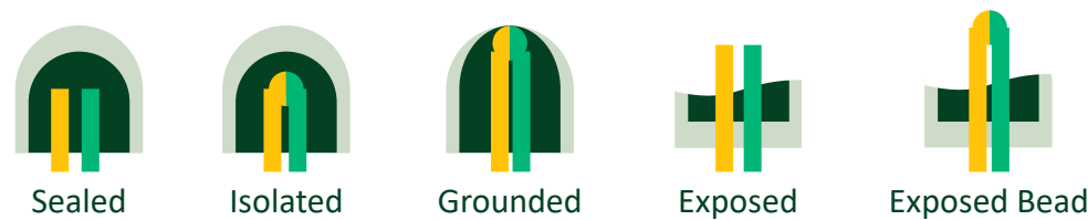
Figure 7. Options for Thermocouple Sheathing
