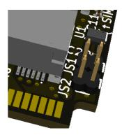
Sierra Wireless EM9190, EM9191, EM7690 defaults to PCI Express data interface. To activate usage of USB2/USB3 data interface instead, assemble jumpers on the JS1 and JS2 pin-headers.
