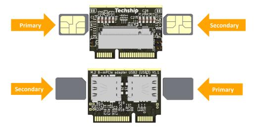
The primary (SIM1) SIM card holder is connected to the primary SIM interface in the M.2 socket. It is also interconnected in parallel with the primary SIM signals from the miniPCle edge connector through zero-ohm resistors.
