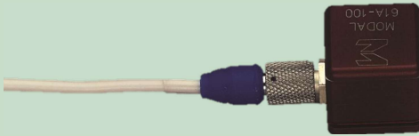
Figure 2. Accelerometers are versatile sensors used for high or low frequency vibration as well as shock
