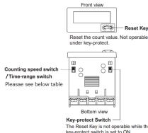
The Reset Key is not operable while the key-protect switch is set to ON.
