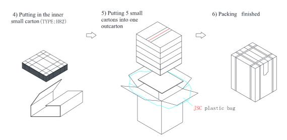
Note: 4 pcs in a tray, 7 trays in a inner carton, 5 inner cartons in a out carton, so 4x7x5=140pcs/Outcarton
