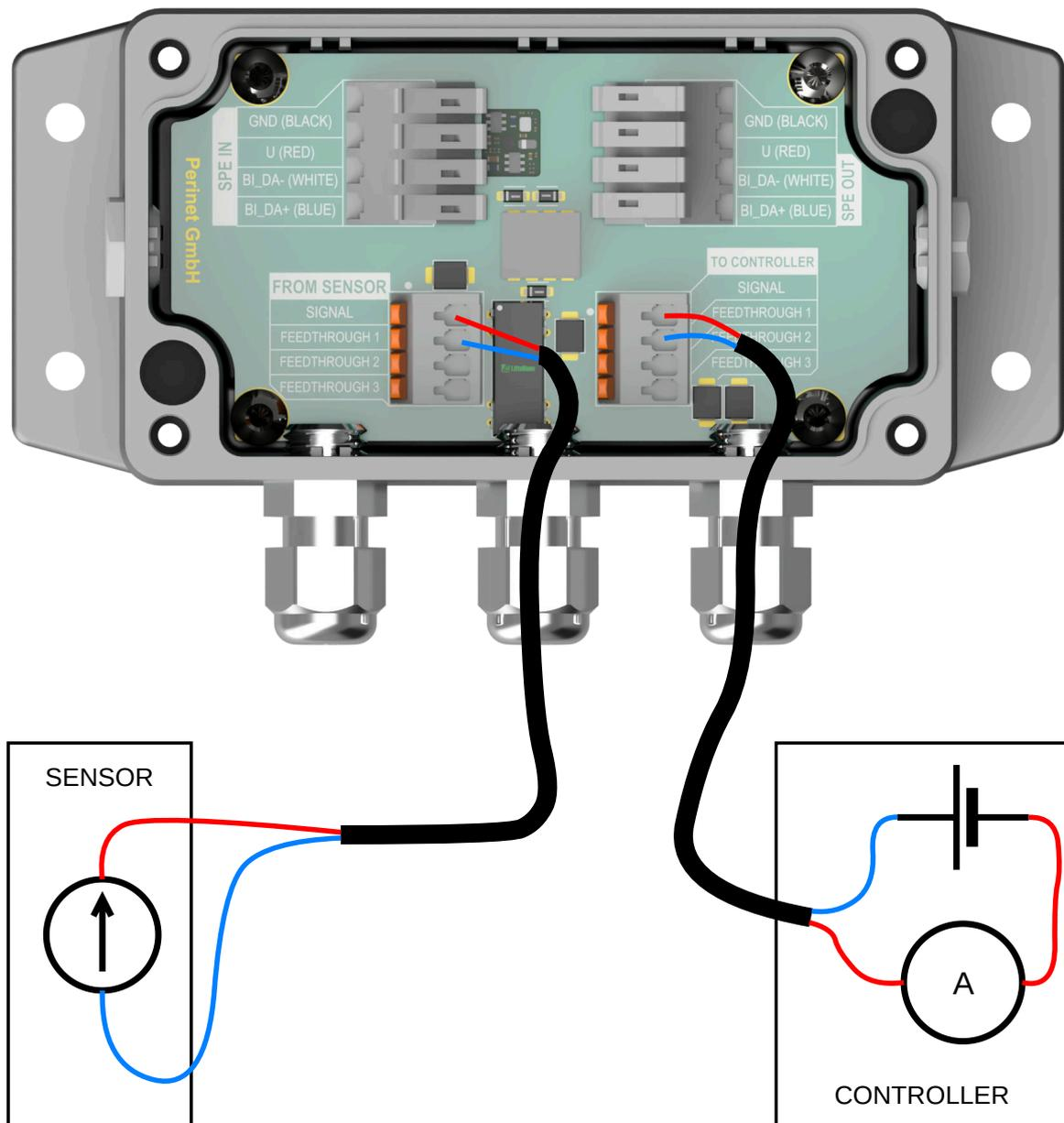
Figure 11: 2-wire sensor wiring
