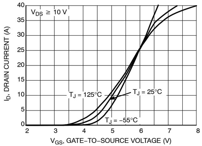
Figure 2. Transfer Characteristics
