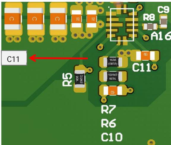
SS time is set at default of 1.4 msec. Adding a small MLCC capacitor between REF and RTN can extend the soft start time.
